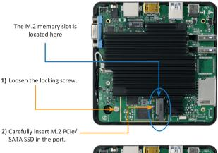
Press the M.2 PCle/SATA SSD into a horizontal position.
